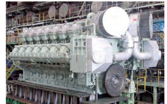
DU-S.E.M.T.Pielstick 14PC4.2BV 18,550kW at 430min -1
